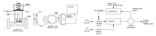
The actuator is used to move the valve stem. They are usually air (pneumatically) or electrically driven. The controller calculates the size of the change to the valve internal passage to bring the flow to the desired rate.
