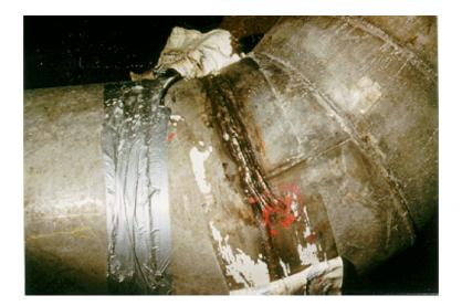
Figure 3. External repairs made to fatigue cracking which initiated at an incompletely penetrated root in a paper machine stock line weld. Such external repairs are temporary as fatigue cracking will persist if root imperfections and cyclic loading remain. Note that the cracking has diverged into the base metal.
